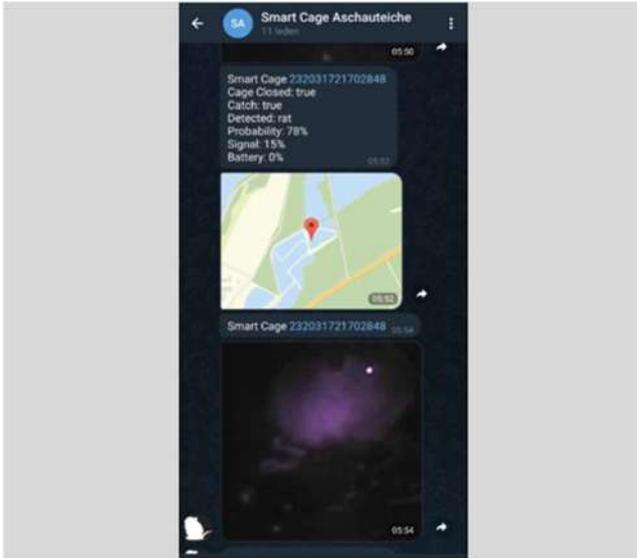
Figure 18: Screenshot of a notification of a coypu catch via messenger service to the smartphone of the trapper.
