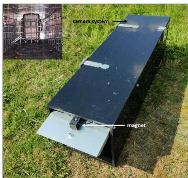
Figure 15: Composition of the prototype of the selective life traps with electromagnet at the door and image recognition system in the rear part of the trap. Inserted picture: image recognition system in the trap.
