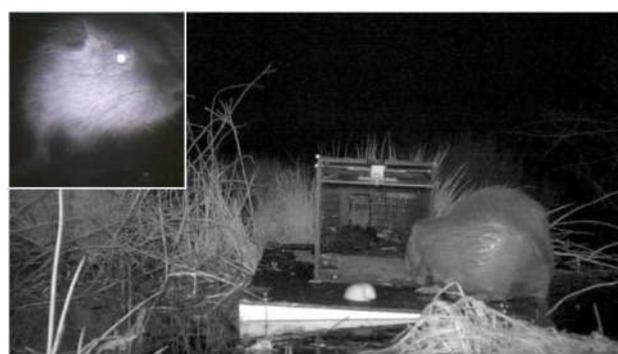
Figure 17: A coypu enters the smart life trap. The inserted picture shows an image taken of the animal by the camera inside of the trap. The image is directly analyzed and classified by the algorithm.
