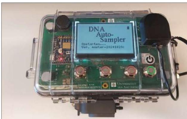
Figure 9: eDNA autosampler for automated water sampling.
