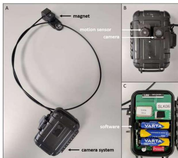
Figure 16: Components of the image recognition system. (A) The camera is connected with the electromagnet, which can be connected to the door of the trap. (B) Frontal view of the camera. (C) Camera system and mini computer from inside.
