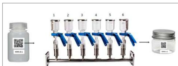
Figure 11: Processing of the water samples. The water from the plastic bottle is filtered and the filter paper containing the eDNA is further processed.
