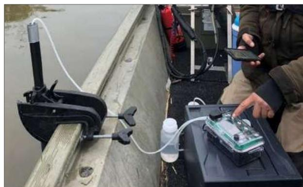
Figure 10: Water sampling via eDNA autosampler from a boat. The water samples run through a plastic tube and are collected in a plastic bottle.
